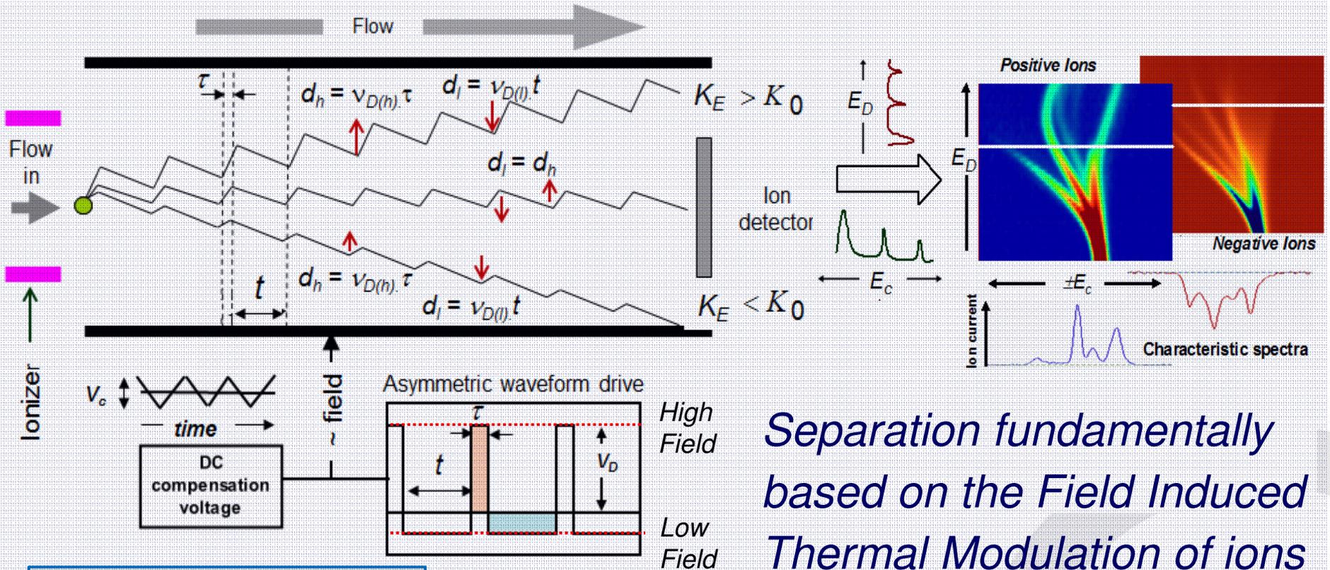
*Separation fundamentally based on the Field Induced Thermal Modulation of ions in the Ion Separator*
