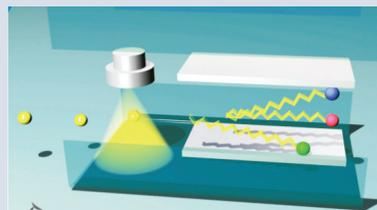
Gas atoms enter the sensor and are ionised with a radioactive source
