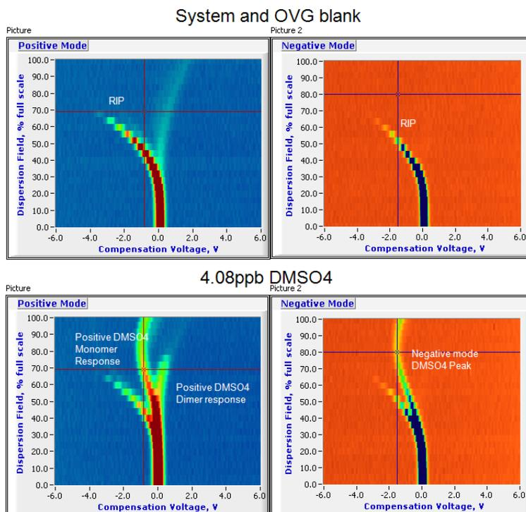
**Figure 4 Comparison of Lonestar blank matrices (top) against a 4.08ppb DMSO4 response (bottom). The blank spectra show the positive (blue) mode RIP made up of hydronium ions and the negative mode (red) RIP response from hydrated oxygen molecules. Peaks caused by DMSO4 are clearly visible in both the positive and negative modes of the Lonestar spectra.**
