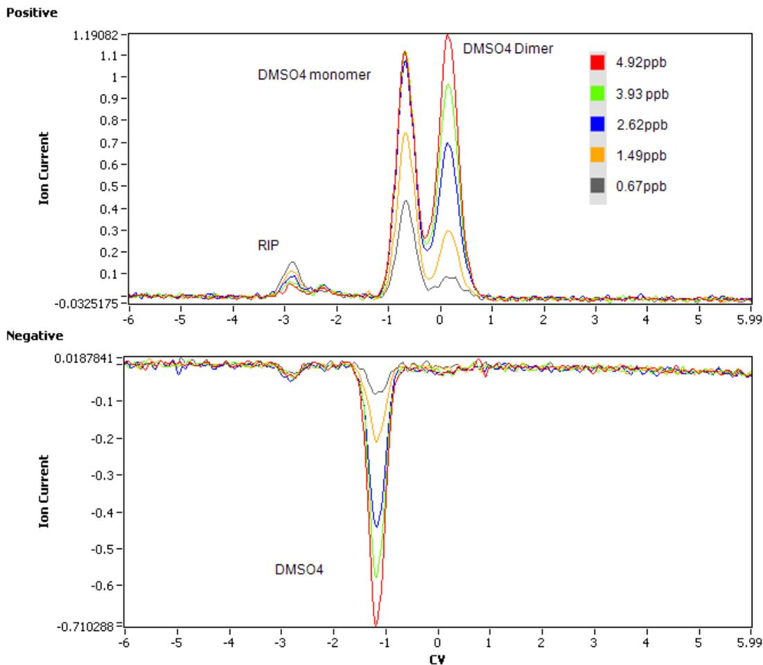
**Figure 6 Example overlaid CV spectra of DMSO4 at various concentration levels (see legend)**
