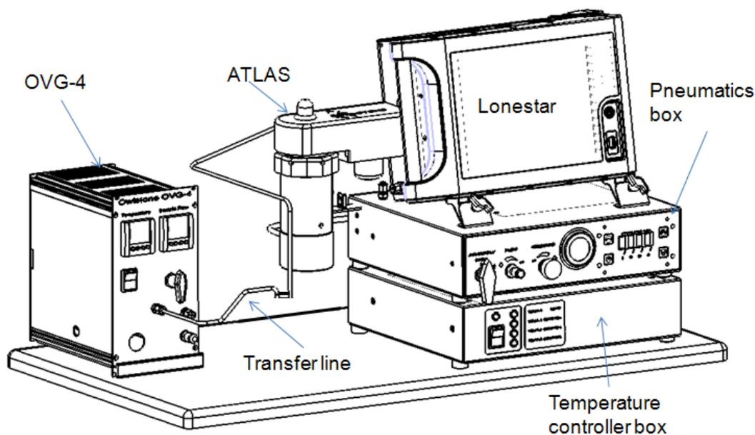
**Figure 3** Experimental set-up, including the Owlstone vapor generator which housed the DMSO4 permeation source at 50°C. The OVG-4 was connected to the Lonestar via the at line sampling module (ATLAS)
