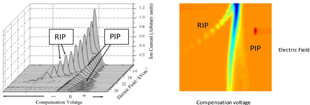
**Figure 16 Two different examples of FAIMS dispersion field matrices with the same reactive ion peaks (RIP) and product ion peaks (PIP). In the waterfall plot on the left, the z axis is the ion current; this is replaced in the right, more frequently used, colorplot by color contours**
