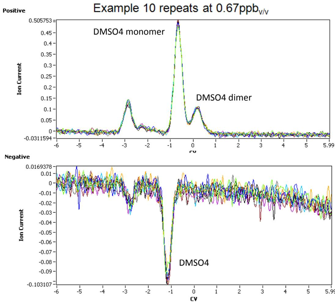
**Figure 5 Example overlaid CV spectra from 10 repeated DMSO4 measurements at 0.67ppb.**
