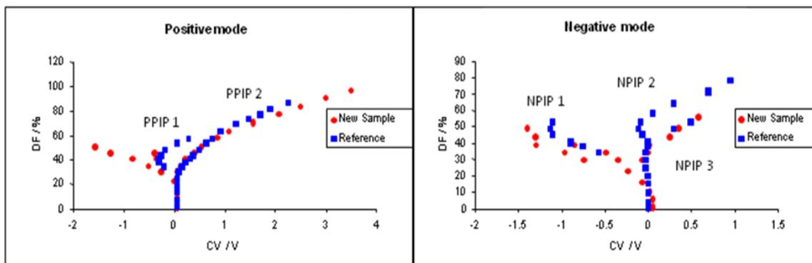
Figure 18 Comparison of two new DF plots with the reference from Figure 10. It can be seen that in both positive and negative modes there are differences between the reference product ion peaks and the new samples
