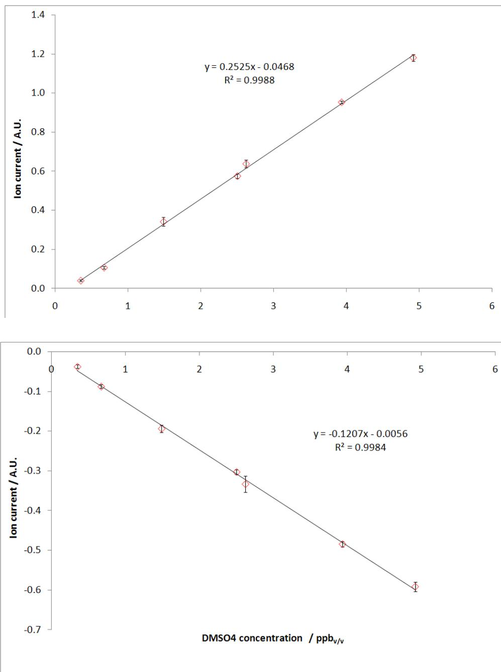
**Figure 7 DMSO4 calibration using the positive mode dimer ion (top) and Negative mode response (bottom). Standard error bars are where n=10**
