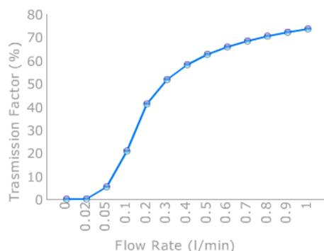
**Figure 9 Flow rate vs. ion transmission factor**
