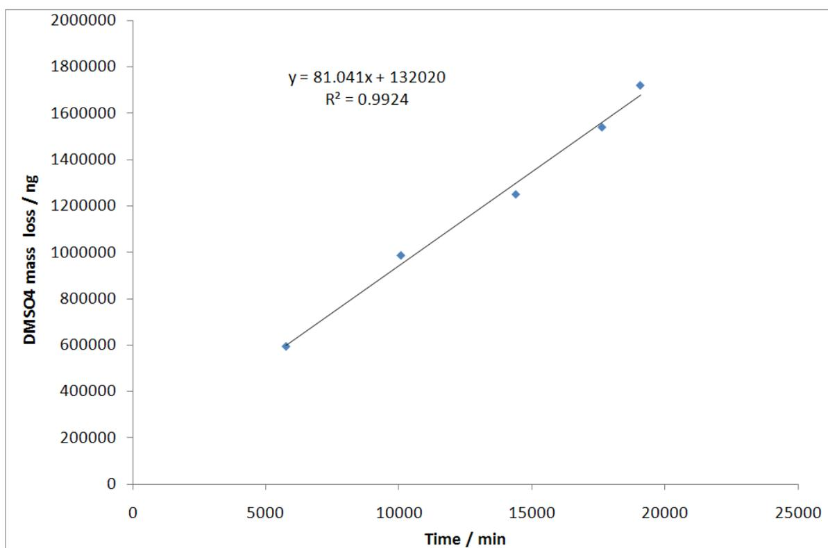
**Figure 2 DMSO4 permeation source calibration, where the slope of the regression line gives a permeation rate of  $81 \text{ ng min}^{-1}$**
